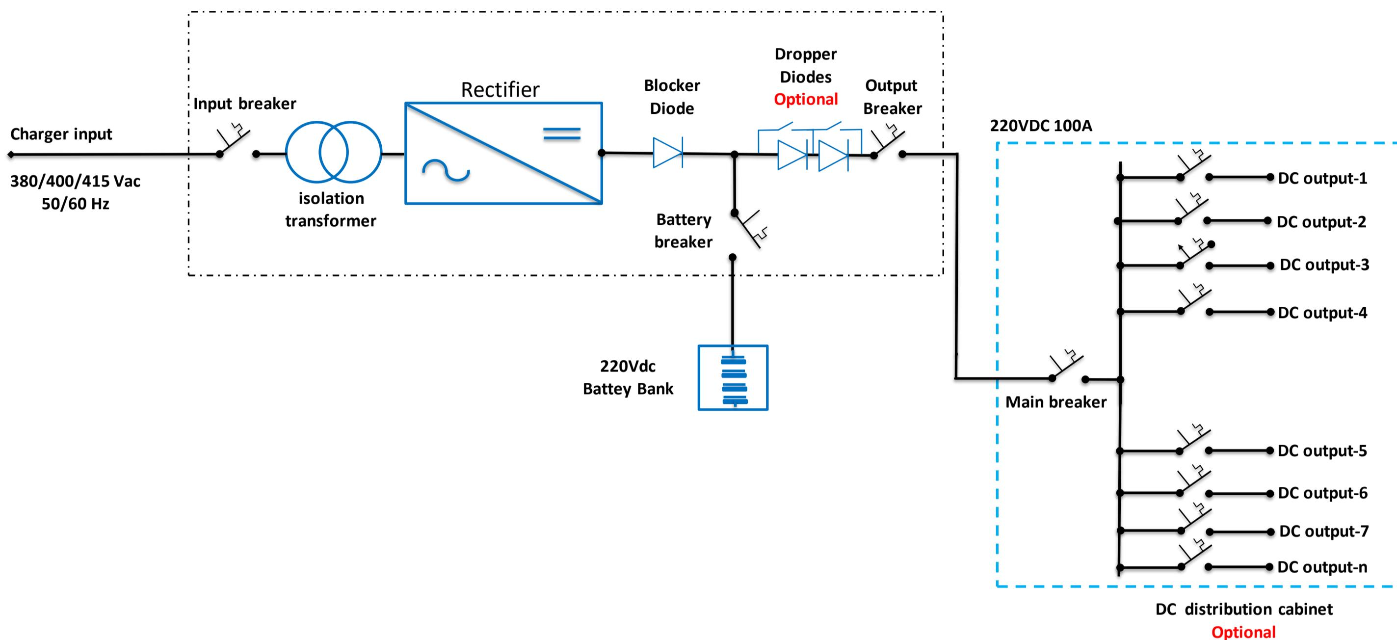
General Redundant Connection Line Diagram
