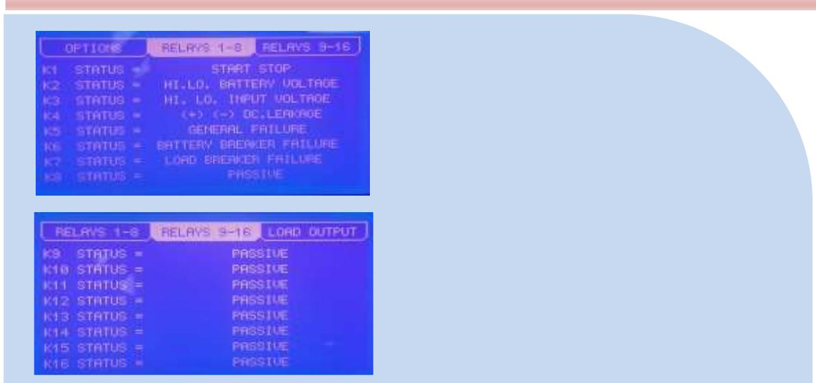
Programmable 2\*8=16 Scada Dry Relay Contacts
