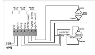
It is used in places with 2 shutters. Button 1 of the controller is loaded to UPS, button 2 is loaded to the receiver unit.
