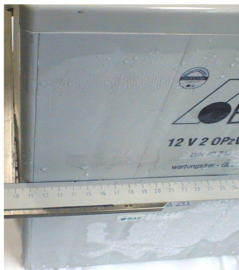
Figure 29 – Picture of test sample during low temperature discharge test: The side walls bulge by about 4 mm.
