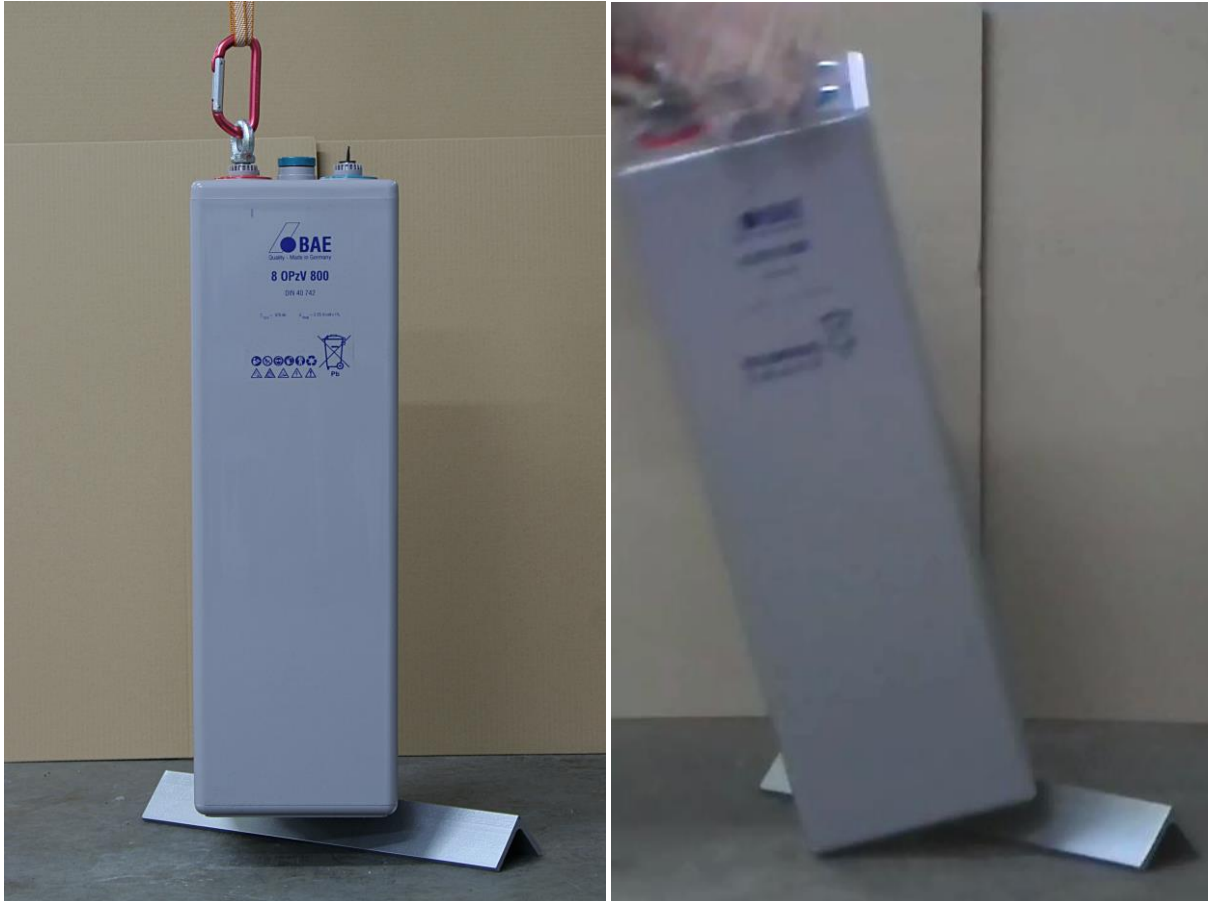
Figure 27 – Test set-up for the drop on one corner.
