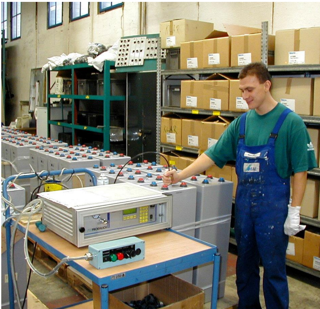
Figure 32 – Measurement of tightness with over pressure.
