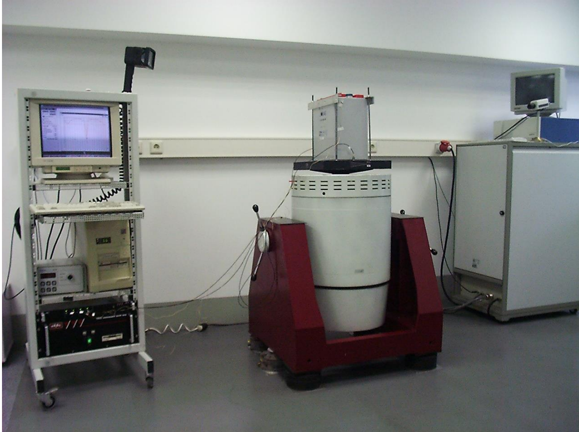
Figure 17 – Test configuration of OPzV block battery for mechanical stress.
