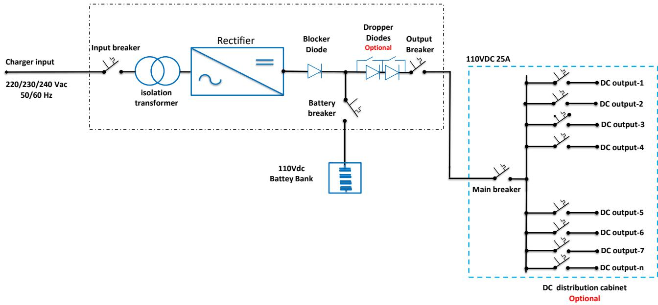
General Redundant Connection Line Diagram
