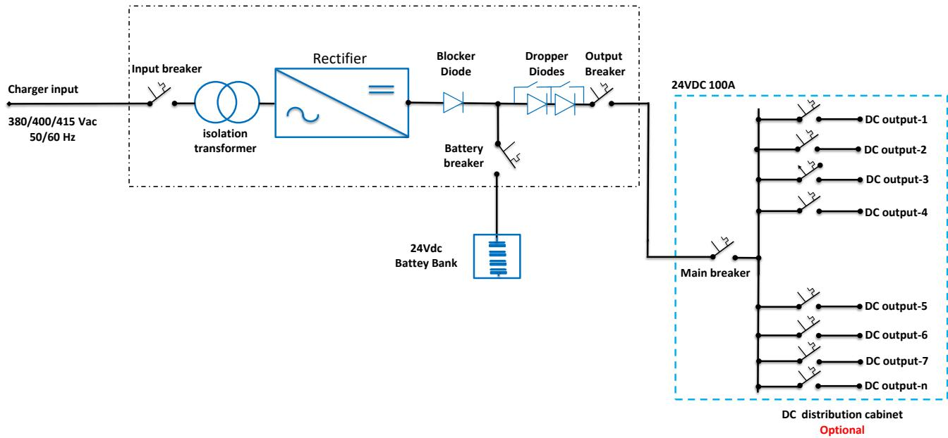
General Redundant Connection Line Diagram
