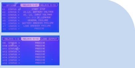
Programmable 2\*8=16 Scada Dry Relay Contacts
