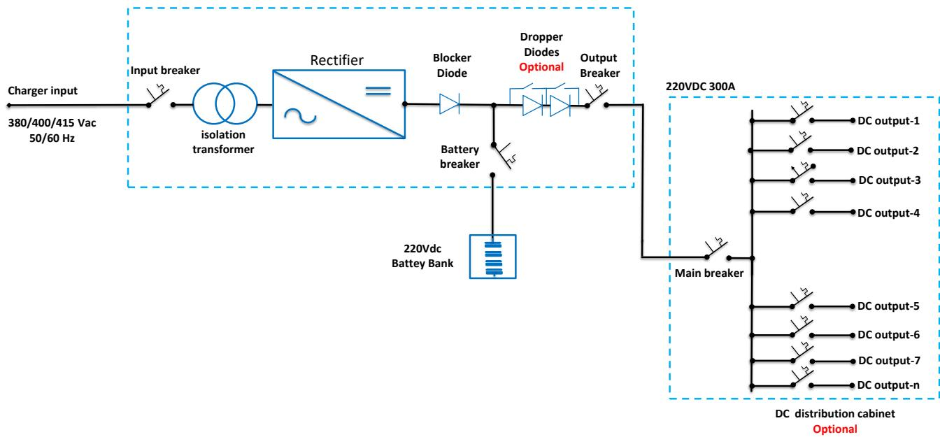
General Redundant Connection Line Diagram
