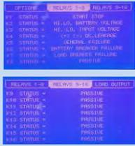
Programmable 2\*8=16 Scada Dry Relay Contacts
